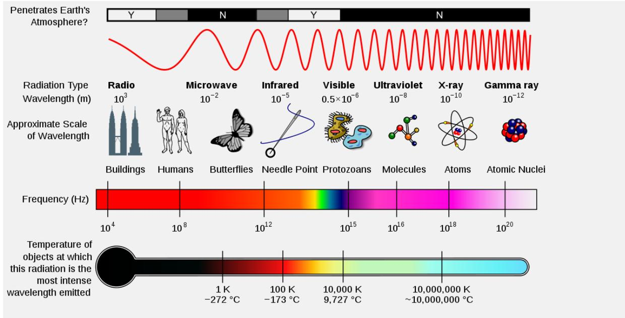
The entire electromagnetic spectrum is much more than just visible light. It encompasses a range of wavelengths of energy that our human eyes can't see. Credit: NASA (via Wikipedia)
